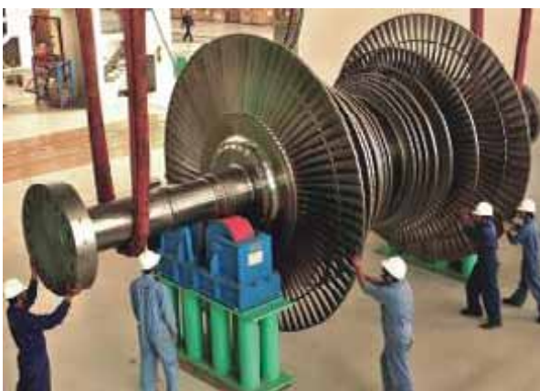
Supercritical turbine under assembly at L&T's Hazira Campus.
