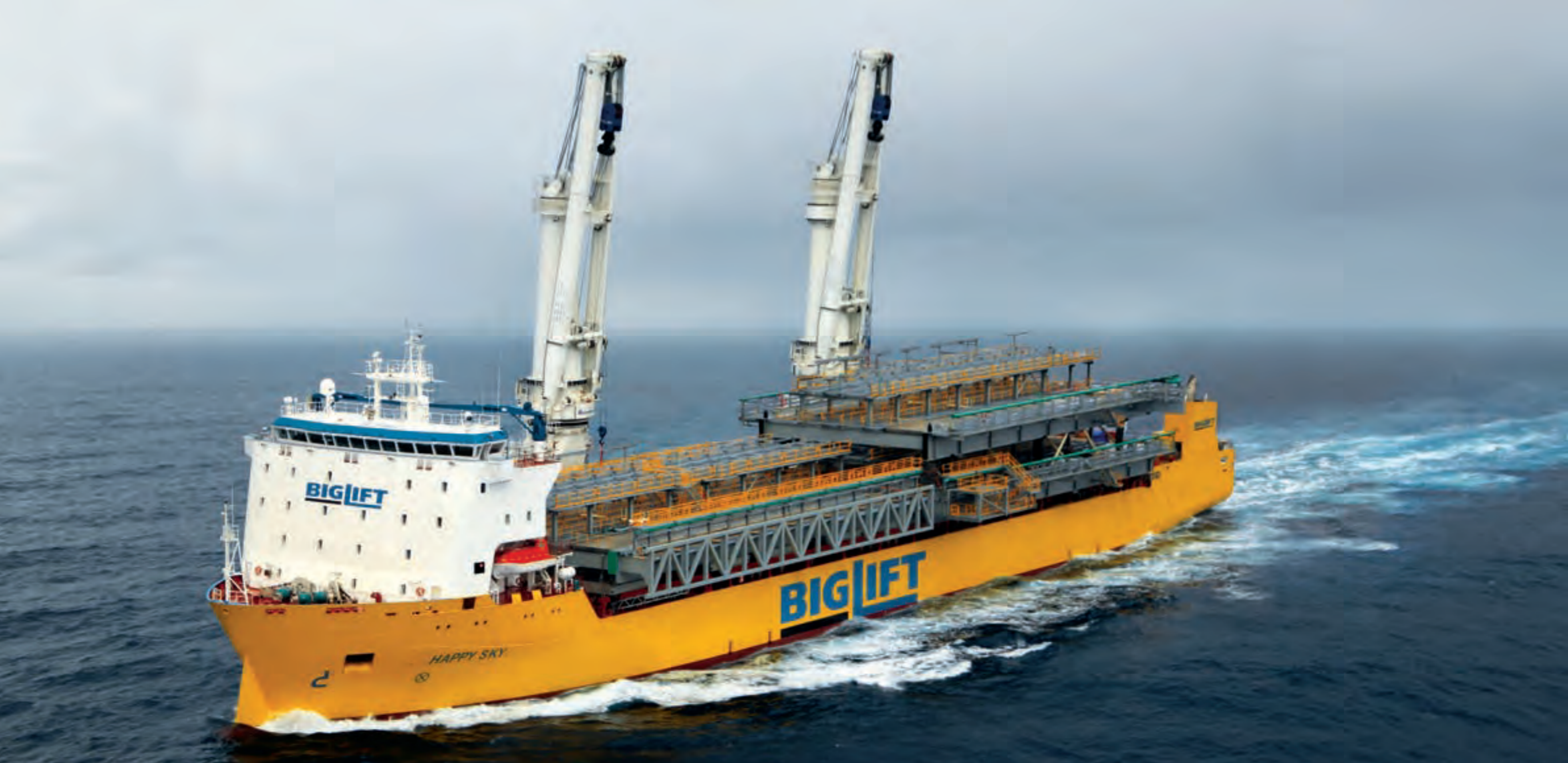
L&T built a 155m-long vessel equipped with two cranes of 900 MT capacity. In addition to commercial ships, the Company focuses on vessels for defence, and undertakes repair and refit.
