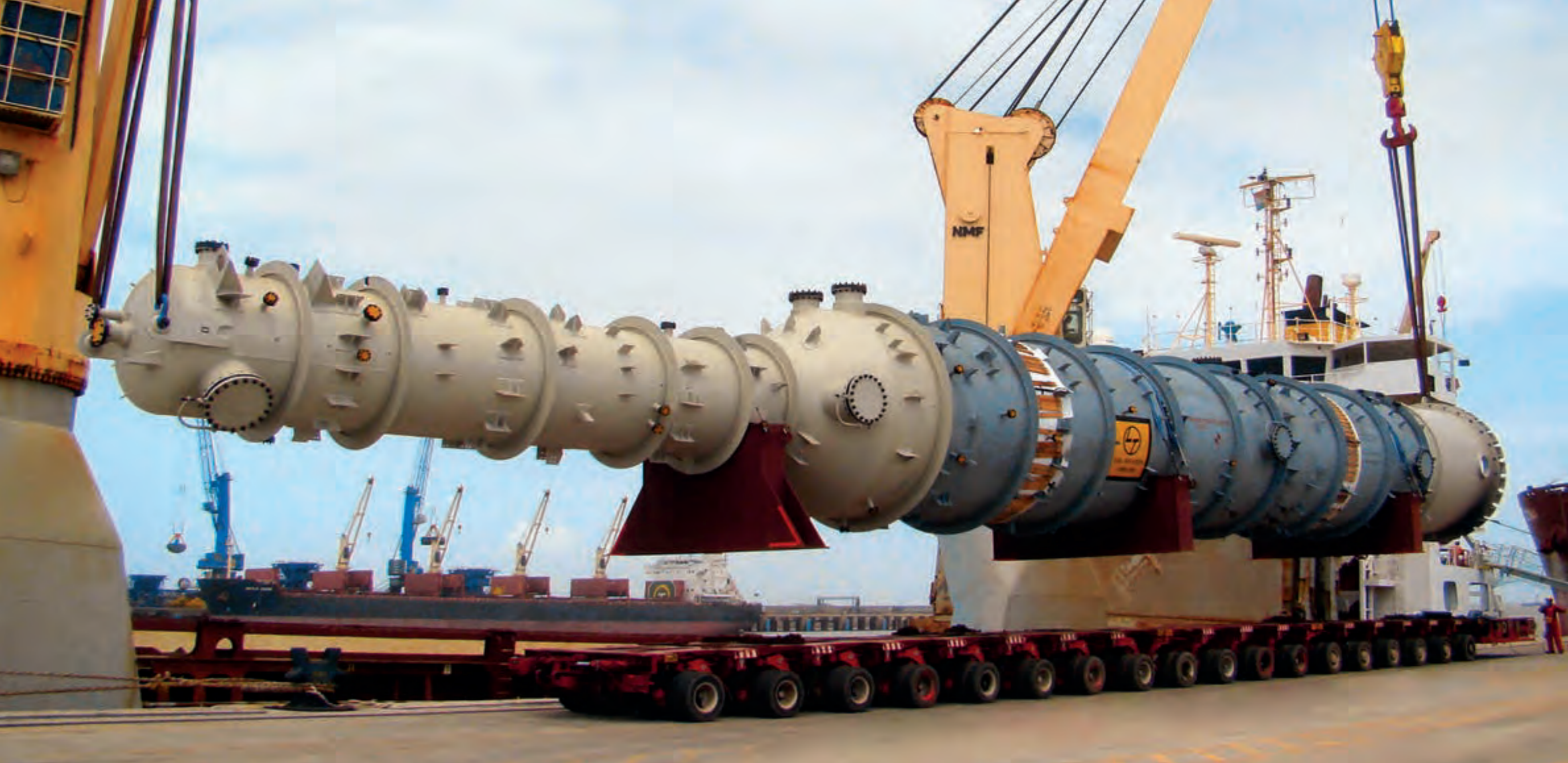
A low-alloy steel HP stripper being shipped from L&T's Hazira Campus to a refinery in Texas. L&T has designed, manufactured and supplied critical process plant equipment to over 40 countries.
