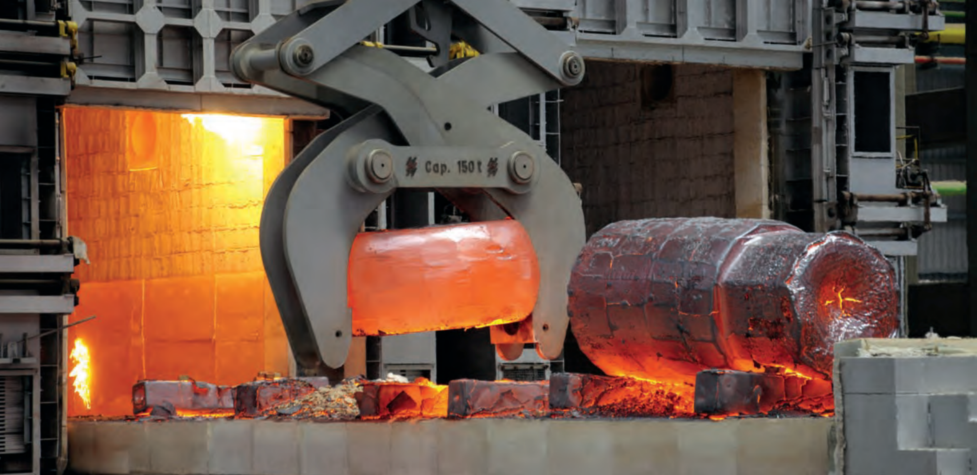
L&T's forge shop at Hazira is among the largest in the world, offering a wide range of finished forgings for the nuclear, hydrocarbon and power sectors. It has the capability to manufacture single-piece forgings of up to 120 MT, and up to 40,000 MT a year.
