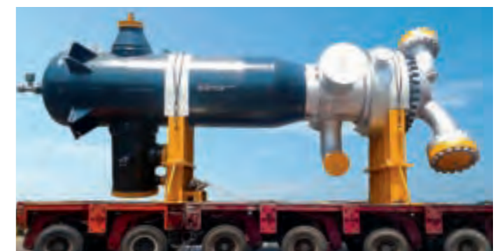
Steam superheater for an ammonia project in the USA.
