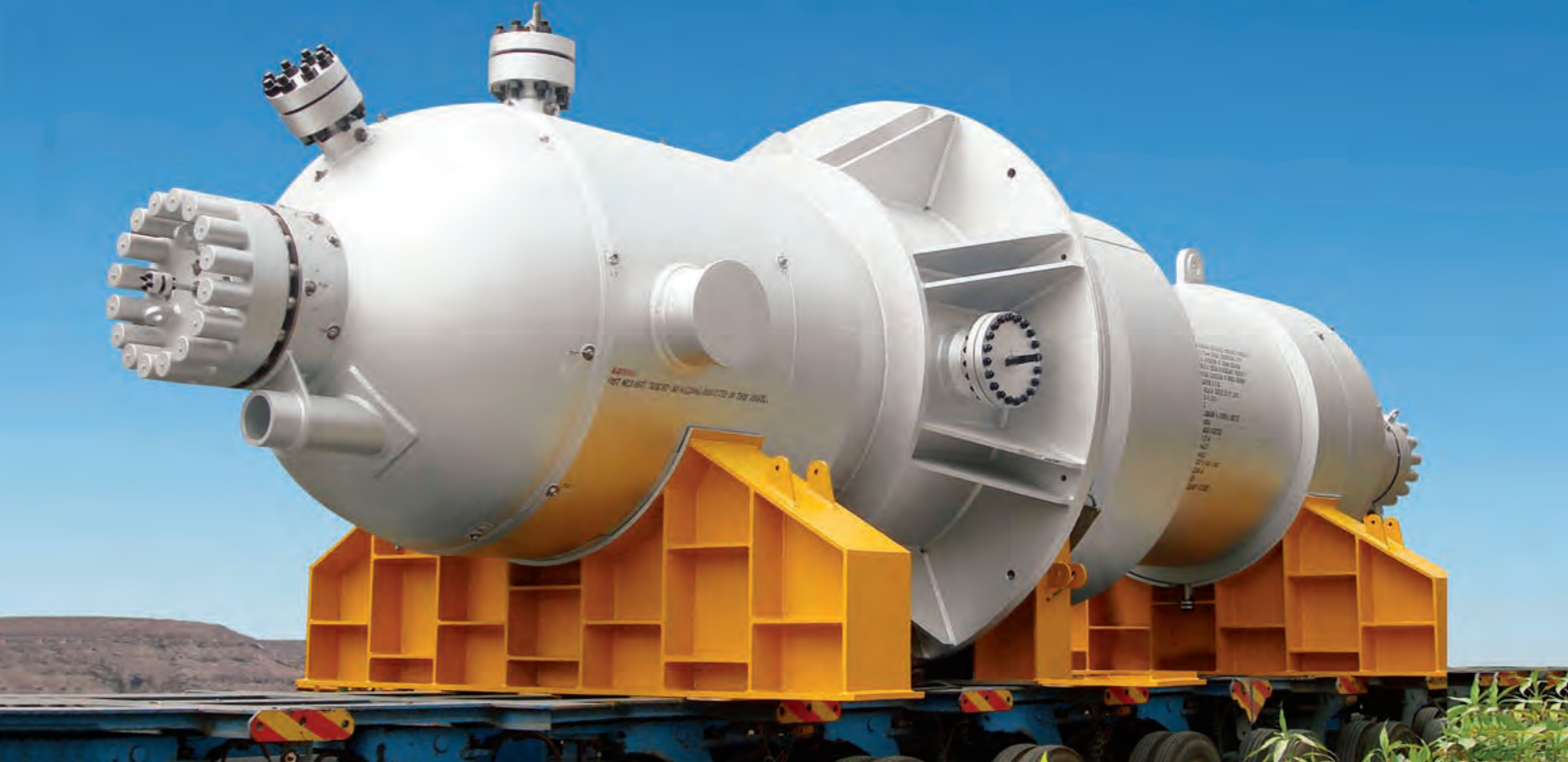
Bi-metallic urea stripper for Saudi Arabian Fertilizer Company. In addition to plant and equipment, L&T has the capability to manufacture and supply complex internals to the specifications of globally renowned process licensors.
