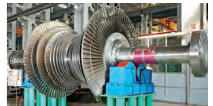
Supercritical turbine being assembled at Hazira Campus.
