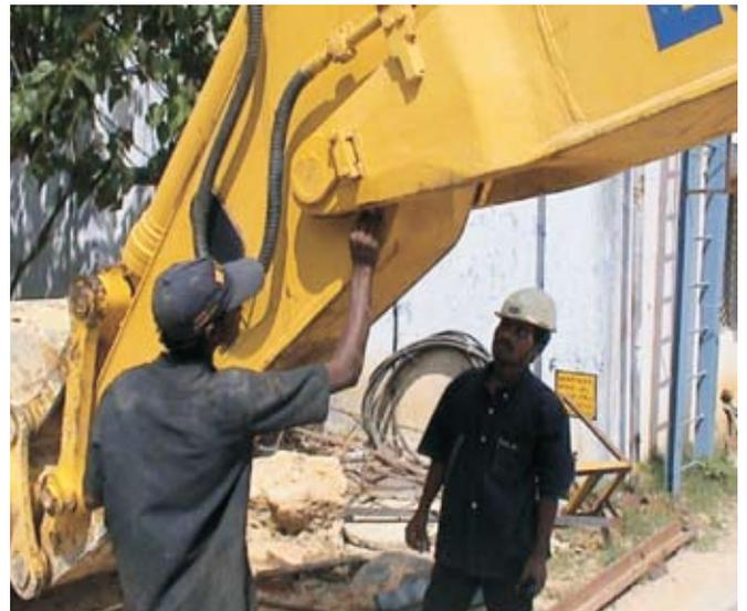
*A well-kept machine at the site, excess grease being wiped after greasing*
