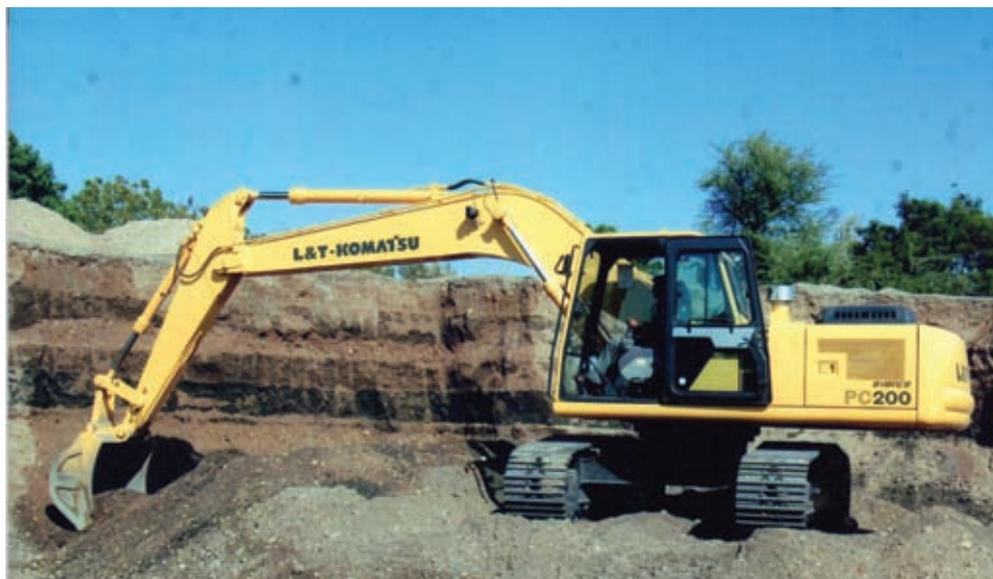
*L&T-Komatsu PC200 Hydraulic Excavator deployed at a site.*
