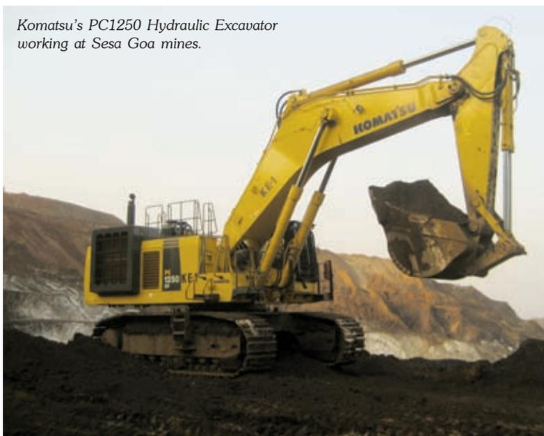
undercarriage is strengthened to provide excellent reliability and durability when working on rocky ground or rock. Sturdy guard shields the travel motors and piping against damage from rocks. Track roller guard (full length) is available as an option.
