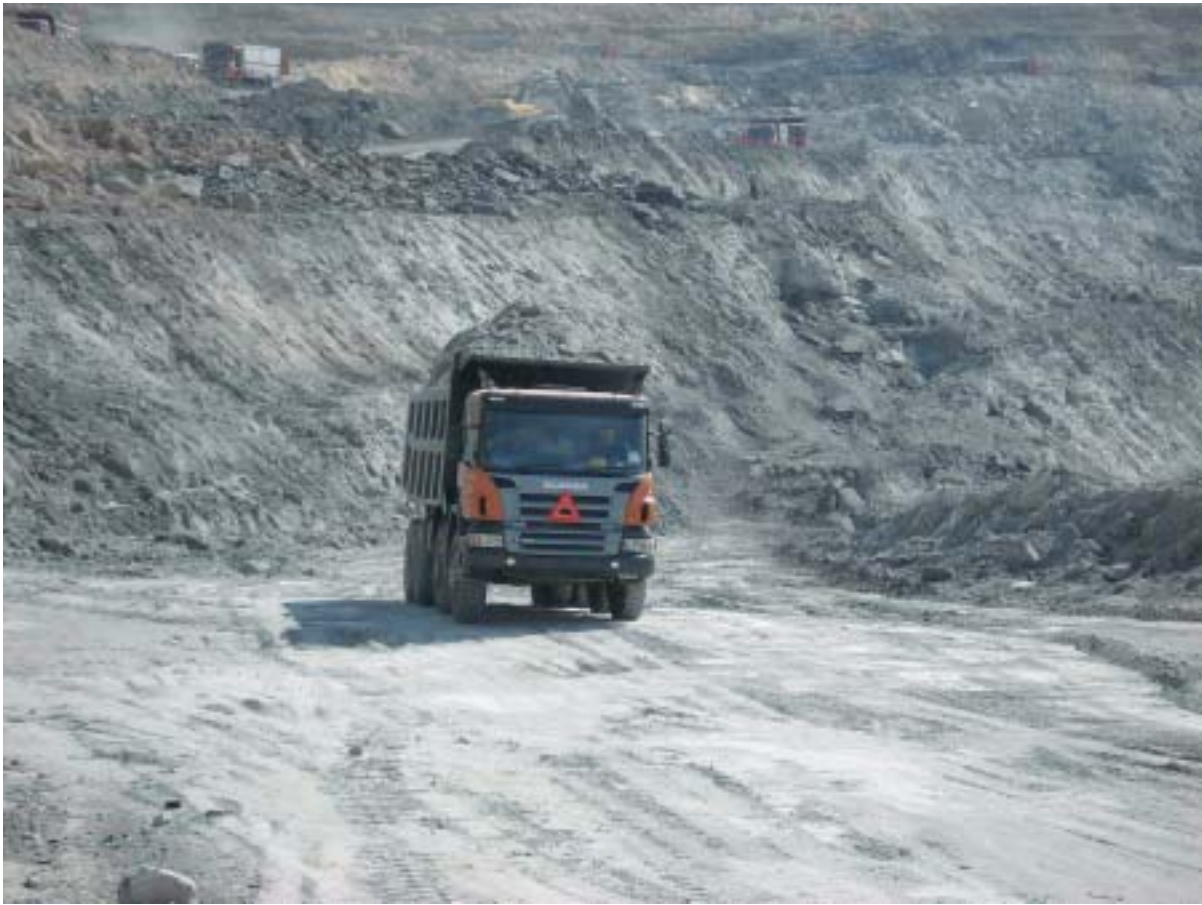
The Scania P380 sets off on the haul road with its load of overburden sandstone
