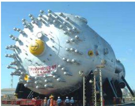
A view of FCC regenerator at L&T's Hazira Works.
