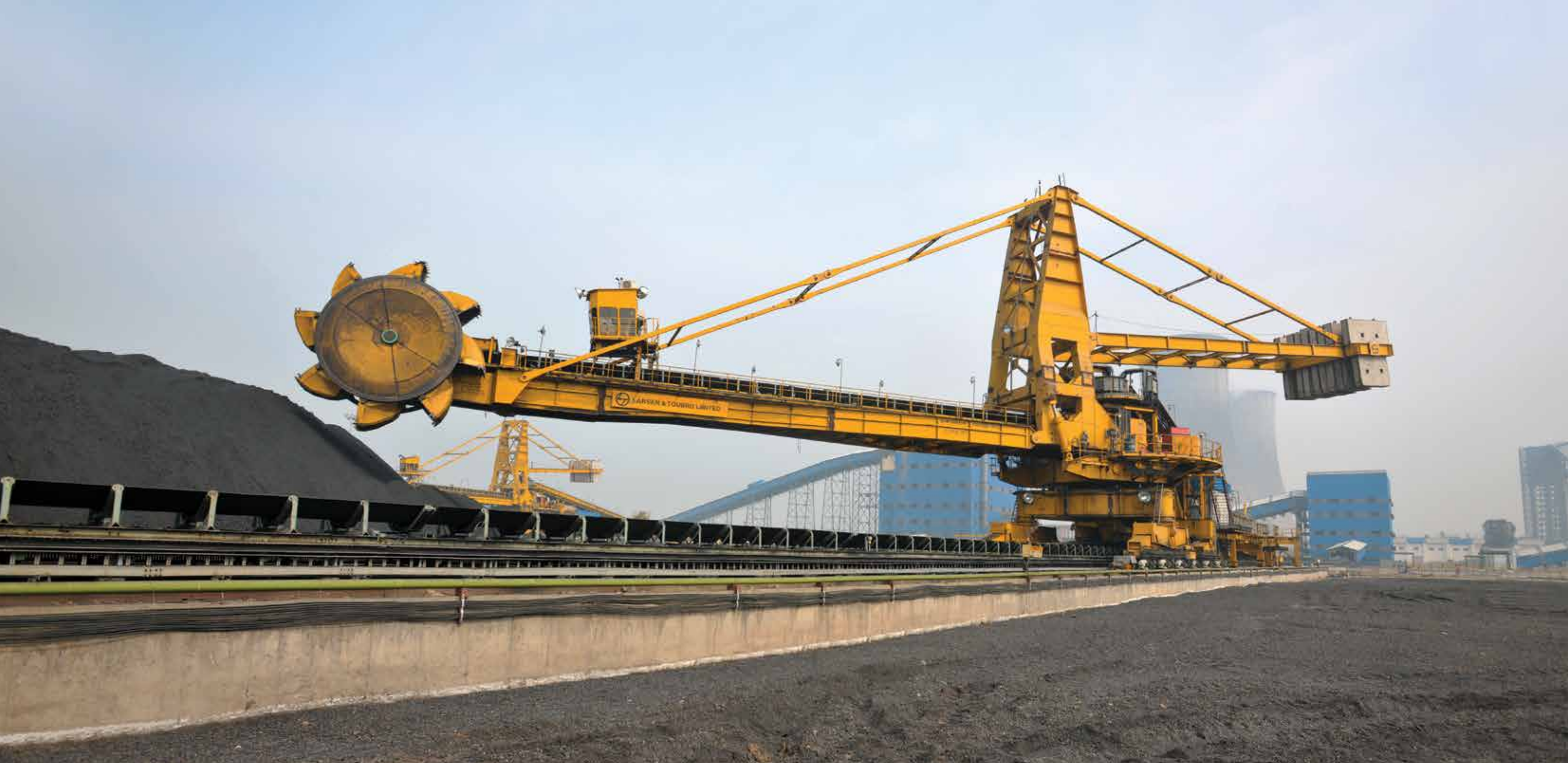
3600 TPH Stacker Reclaimer, Rajpura, Punjab. L&T is a one-stop solutions provider for all bulk material handling requirements for power, steel, mines, ports, cement and other industries.
