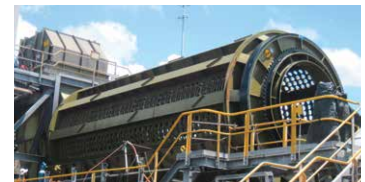
1600 TPH Rotary Breaker manufactured at Kansbhal and supplied to Rio Tinto, Australia.
