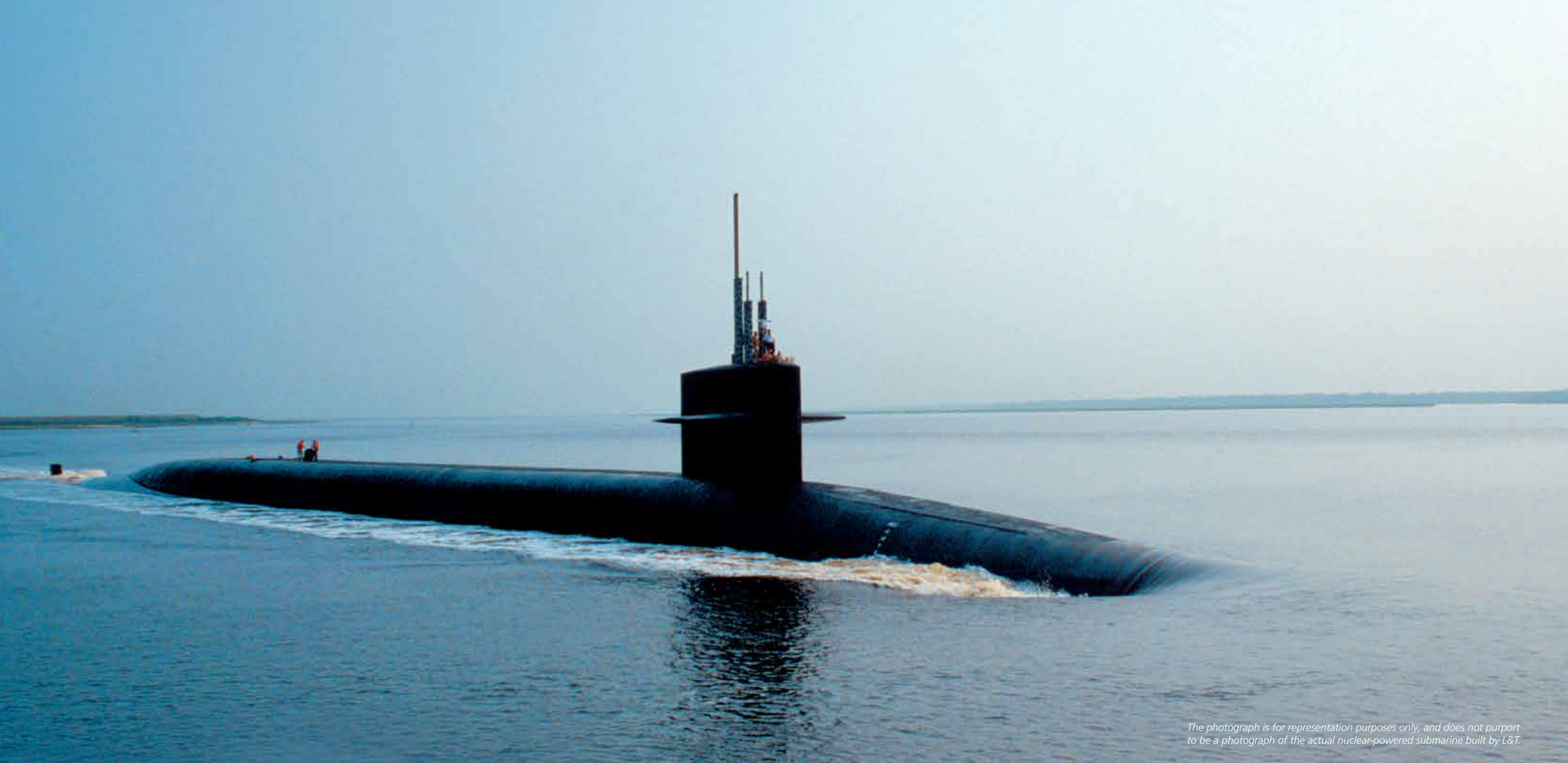
L&T's contribution to INS Arihant – India's first Nuclear Powered Submarine included design engineering, pressure hull, outer hull and structures, special equipment, outfitting – equipment, piping, cabling systems, integration and trials.
