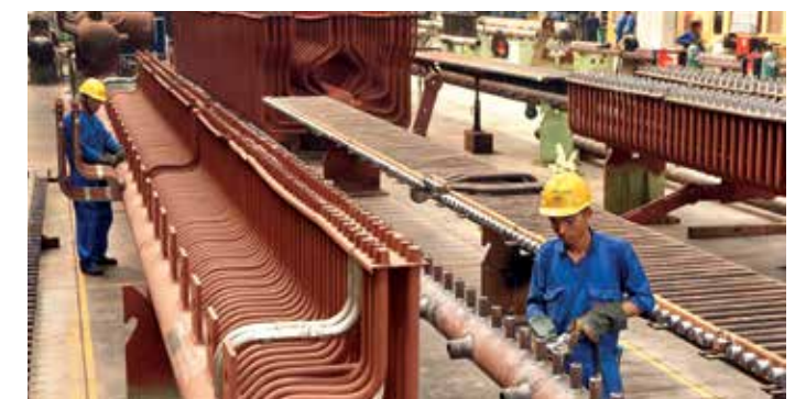
Supercritical boiler made at state-of-the-art manufacturing facilities at Hazira.
