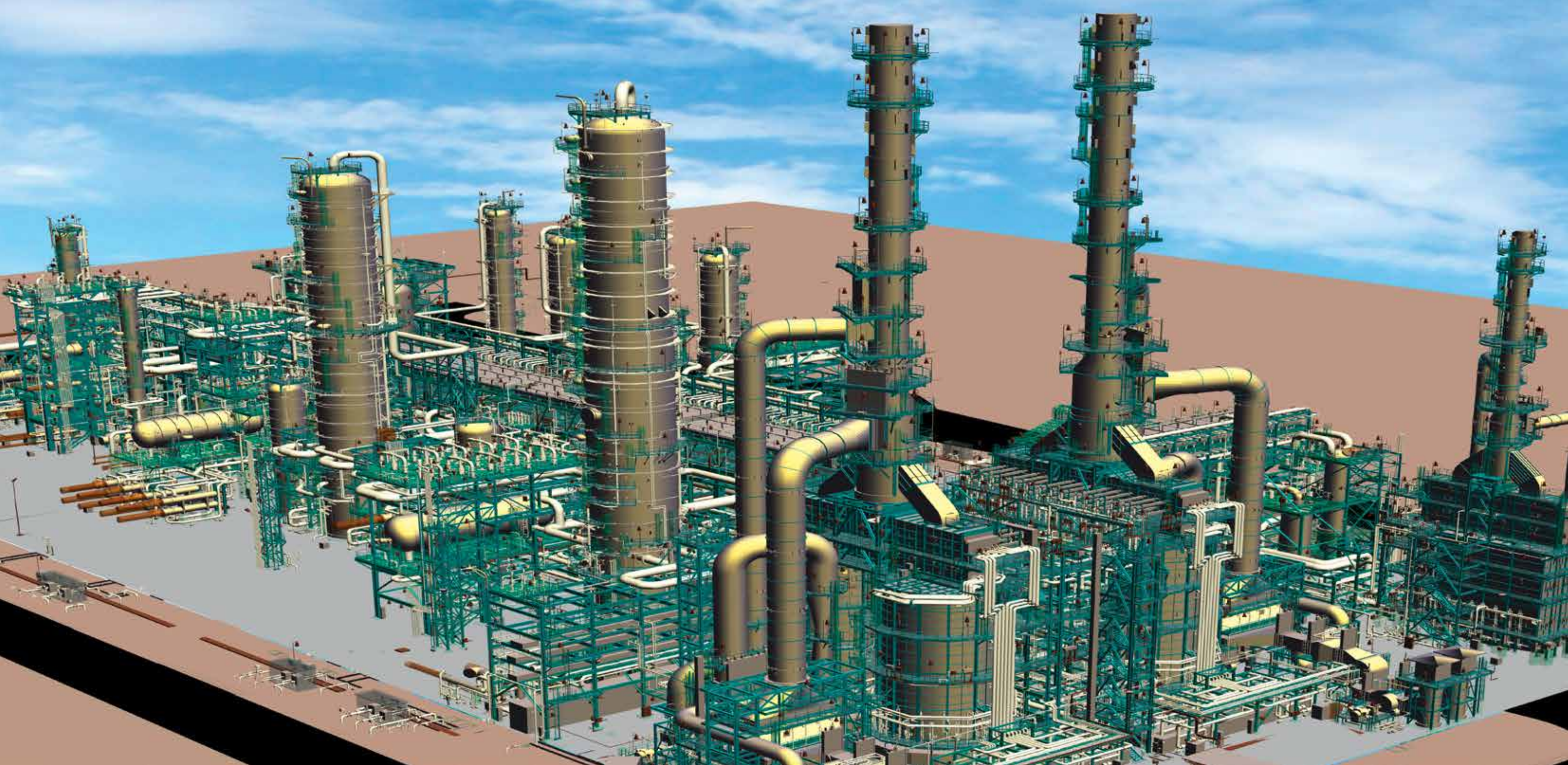
3-D rendering of a petrochemical plant. The Company has engineering centres dedicated to providing detail engineering and FEED services for mid & downstream projects across the hydrocarbon spectrum.
