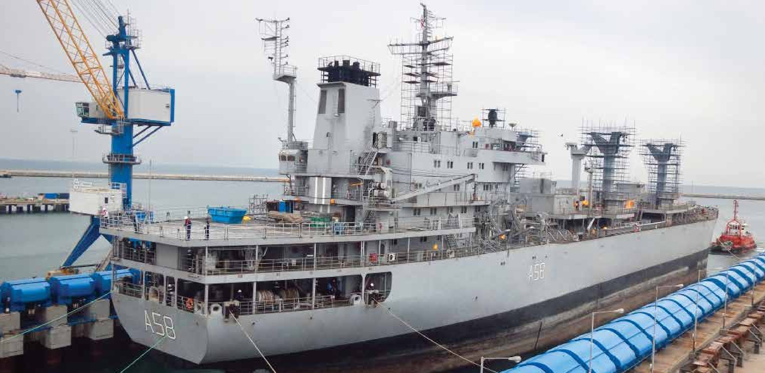
A 28,000 DWT defence vessel on the ship-lift at L&T's shipyard at Kattupalli. L&T offers ship design, building, maintenance and repair services for defence and commercial vessels.
