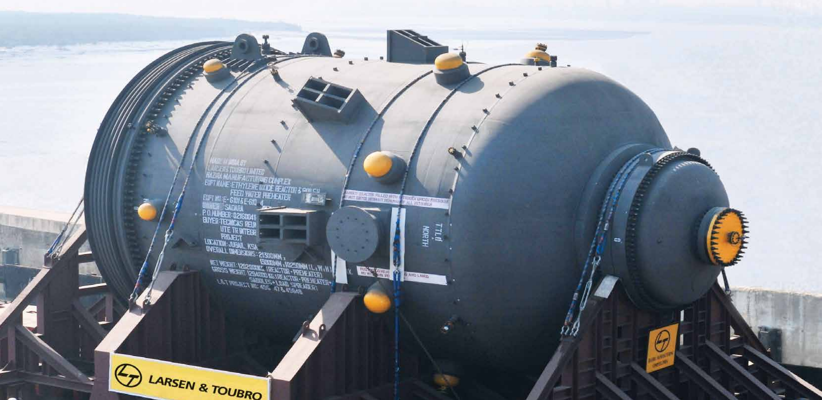
1200 MT Ethylene Oxide Reactor for Saudi Arabia. In addition to plant and equipment, L&T also manufactures and supplies complex internals to the specifications of global process licensors.
