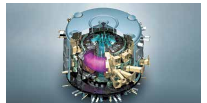
L&T will build the cryostat for the prestigious ITER project. The cryostat will be the world's largest high-vacuum pressure chamber.
