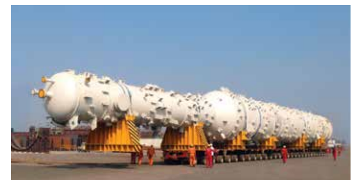
Unsaturated Gas Demethanizer. L&T has designed, manufactured and supplied critical process plant equipment to over 40 countries.
