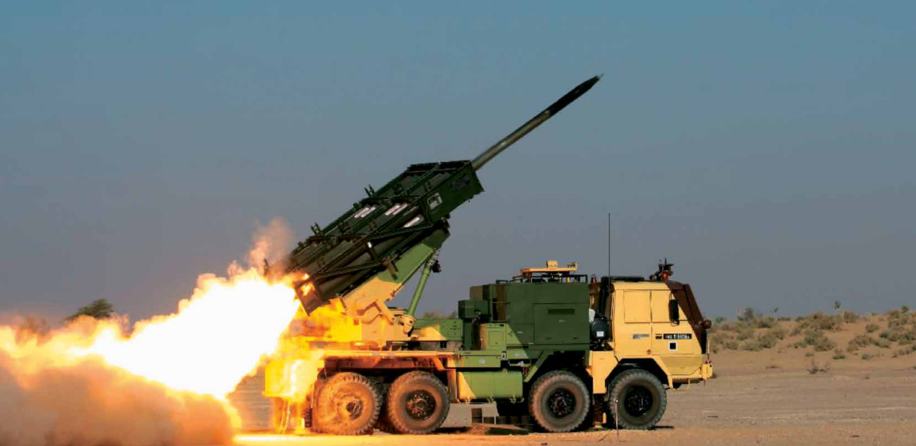
Pinaka multi-barrel rocket-launcher. L&T works closely with defence research organisations to develop and manufacture weapon and missile systems.
