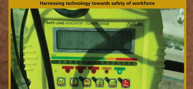
To ensure safety at site L&T's building factories business has installed Safe Load indicator on its tower cranes being used at its major projects.
