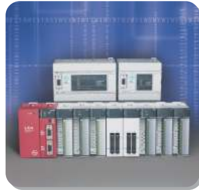
Programmable Logic Controllers (PLCs)
