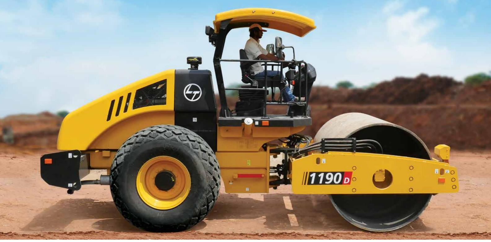
L&T soil compactor, model 1190D. LTCEL manufactures a range of equipment for the construction and mining industry.
