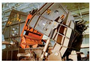
Limestone crusher manufactured by L&T.
