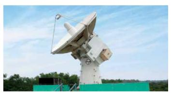
Monopulse tracking radar - one of many indigenous radars and tracking systems developed by L&T.
