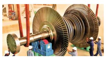
Supercritical turbine being assembled at L&T's Hazira Campus.
