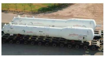
Steam generators for Pressurised Heavy Water Reactors.
