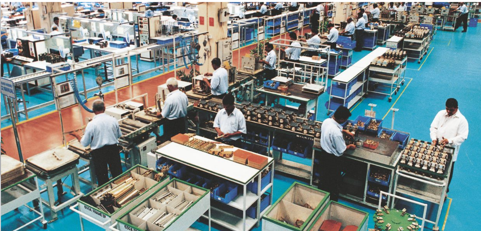
ACB Assembly Shop where over 36000 ACBs are manufactured per year.
