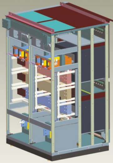
3D Modelling of Switchboard
