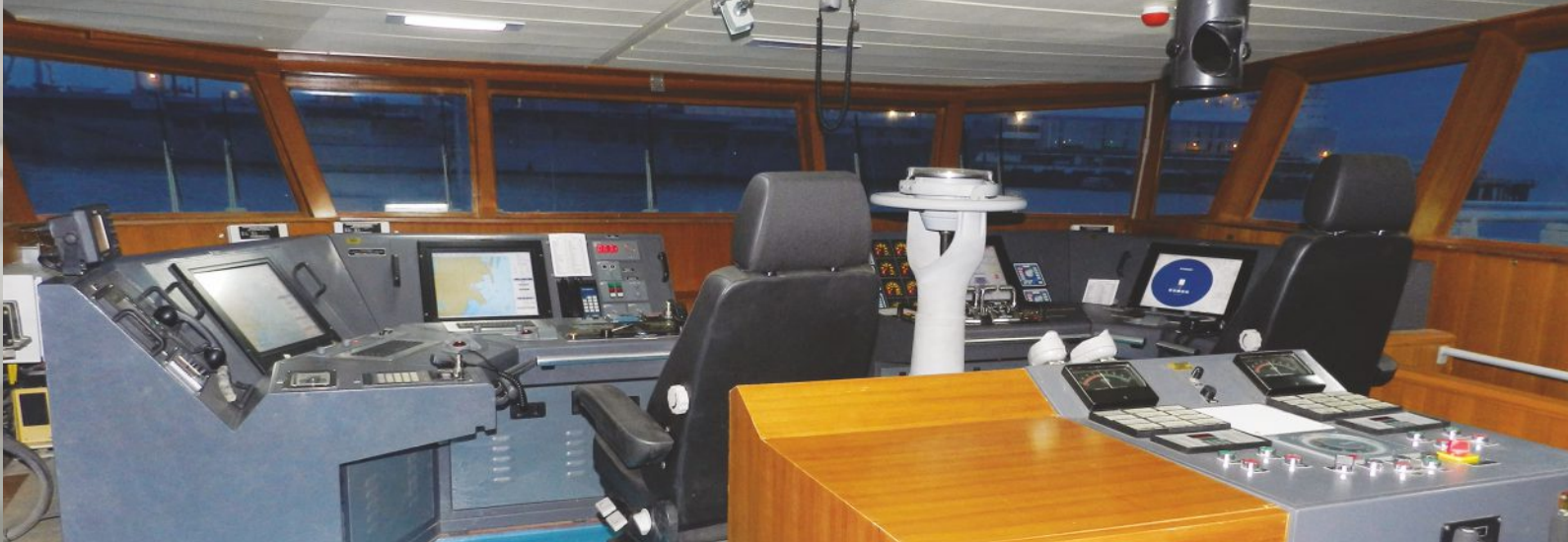
Integrated Bridge System
