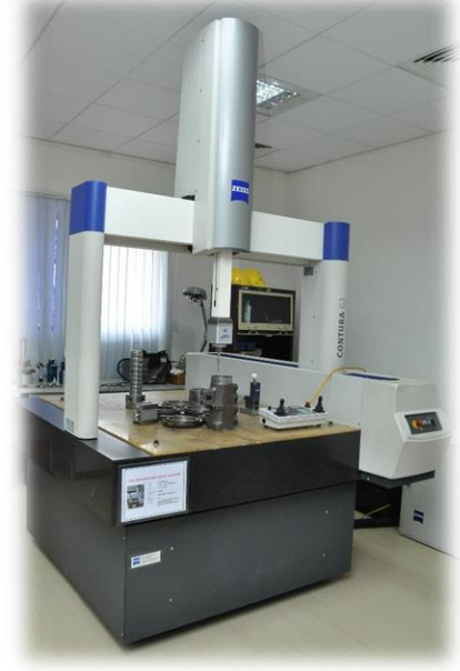
Carl Zeiss Co-ordinate Measuring m/c
