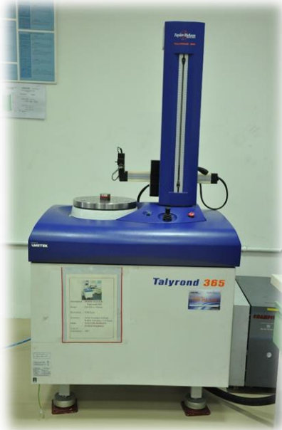
Form tester for Roundness, Cylindricity of super finished parts
