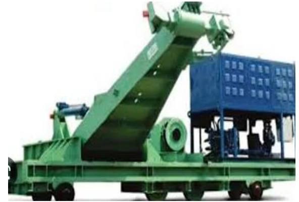
Side Arm Charger Hydraulic Power Pack
