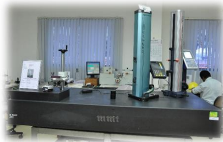
Surface Table 00 Grade for calibration
