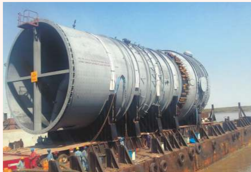
World's largest acrylonitrile reactor is being dispatched to Thailand using roll-on-roll-off jetty at Hazira Manufacturing Complex
