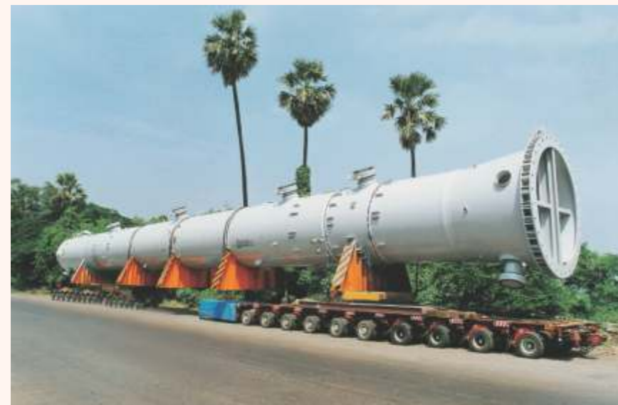
3.3 m dia, 38 m-long Absorber for Burrup Peninsula, Western Australia, for Kellogg JV / Woodside Energy Limited
