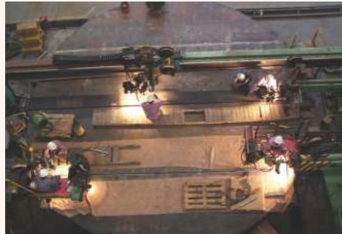
Fabrication of 10 meter diameter, 444mm-thick tube sheet for tubular reactor
