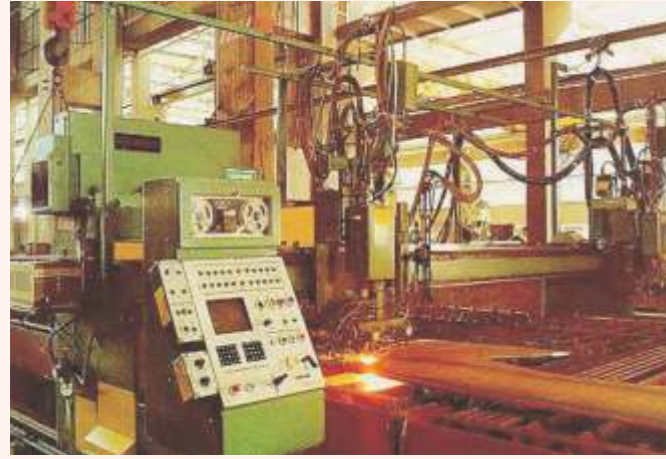
CNC Flame/plasma cutting machine for cutting 450mm-thick alloy steel plates
