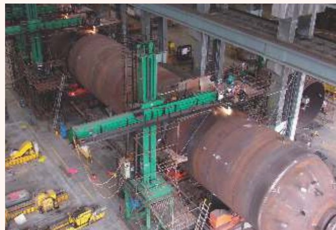
Narrow gap tandem SAW on a thick-walled reactor circular seam
