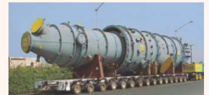
ODC equipment up to 350 tonnes in weight, 7.5 metres diameter and 50 metres in length has been delivered safely over land to remote locations in India.
