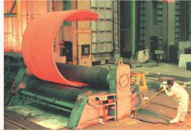
Plate-rolling machine for hot rolling plates 250mm-thick and 4500mm-wide
