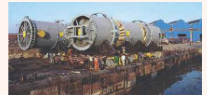
Tubular reactors for China, loaded onto the barge at the roll-on/roll-off jetty at Hazira.
