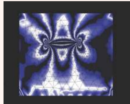
Fracture mechanics evaluation of a crack in a weld joint
