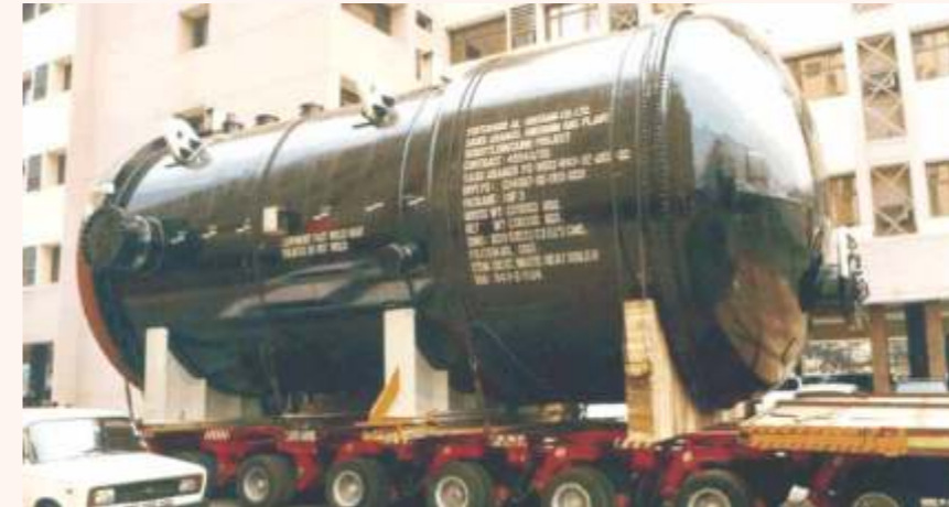
WASTE HEAT RECOVERY BOILERS (for sulphur recovery)
