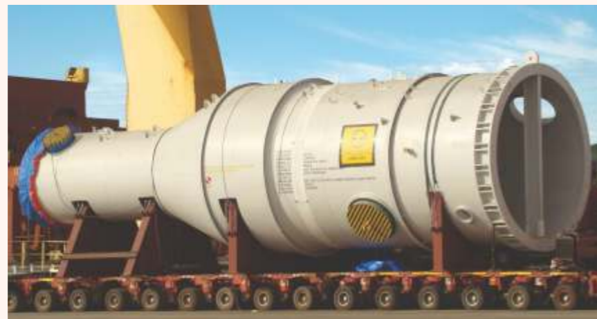
A 180 MT Secondary Reformer supplied to PT Pupuk Kaltim, Indonesia
