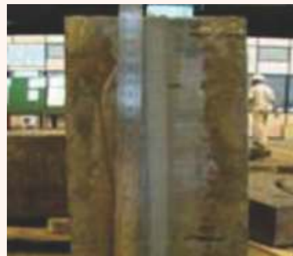
800mm-thick weld joint by narrow-gap SAW
