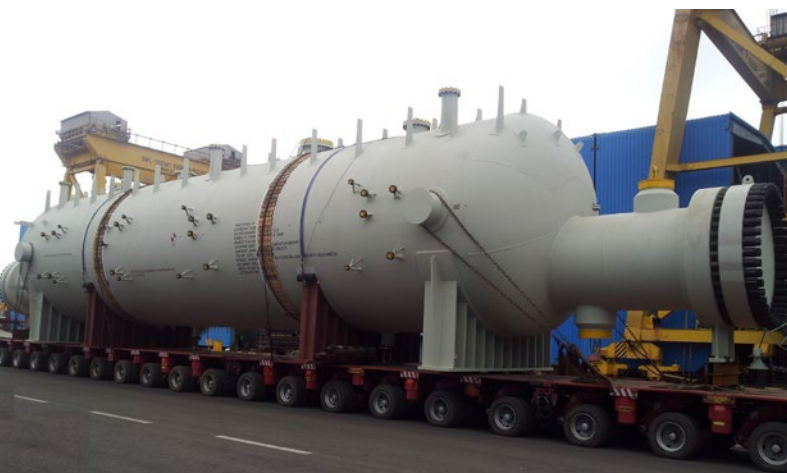
Unitized Chiller weighing 380 MT for a project in Indonesia
