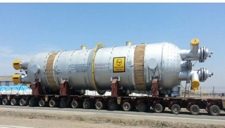
Methanol Converter for Yanchang, China weighing 392 MT
