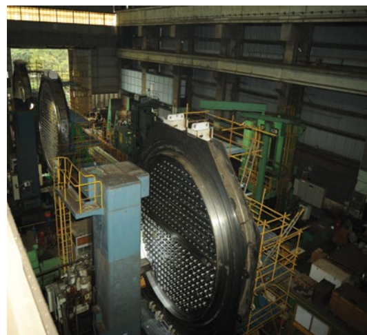
CNC Vertical multi-spindle deep-hole drilling machine. Drilling Depth: 900mm Number of Spindles: 2
