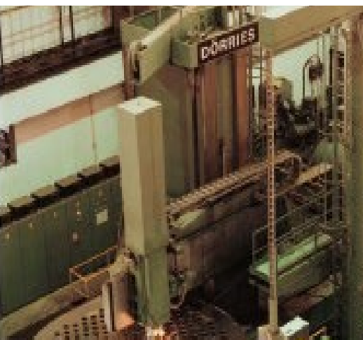
CNC Vertical boring machine Max. Diameter: 12m, Max. Job Weight: 130 MT
